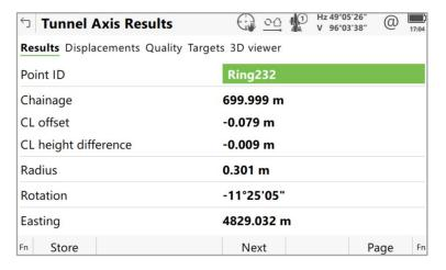
In addition, the as-built attitude (orientation and pitch) of rings can now be calculated relative to the design trajectory (to deliver "lead" and "look up" values).
