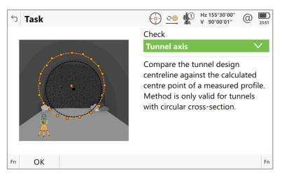
In Leica Captivate v8.30 this method has been enhanced with two additional features. The relationship of the design tunnel axis can now be determined with rotation & shift values from an alignment.
