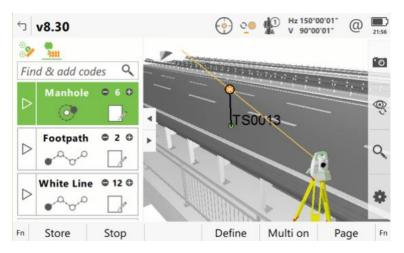
With Leica Captivate v8.30, a new play button on each code box gives a touchscreen user the ability to 'tap to measure'. A single screen tap on the code box will both select that code and trigger a point measurement. This reduces the number of screen taps that are needed for measuring points, allowing to be more productive in the field.
