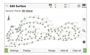
The **Range** option includes several methods to help when needing to select many points, including defining **Start and end points**, or using the 3D viewer to define a **Selection window**.
