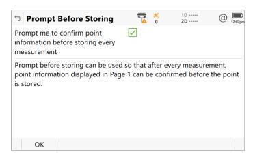
When the **Prompt before storing** setting is activated, after every point is measured in the **Measure** app, the **Confirm Point Information** panel will appear.
