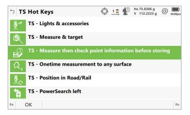
This hot key works independently of the **Prompt before storing** setting, allowing points without a code change to be stored with **F1** or **OK**, if the setting is turned off, but then points that do require a code change or check, can be measured with the hot key.
