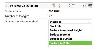
The consistency between all the volume calculation methods has been improved, so that the "from" and "to" are always selected in the same order for every method. This means that the direction of the existing **Surface to surface** method has been reversed.
