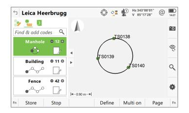
Note that because auxiliary points are used to construct the 3 pt rectangle, 2 pt and 3 pt circles, the line used to represent the shape will not be linked to the measured points within the database. This means that the geometry of the line will not be editable once the shape is completed.
