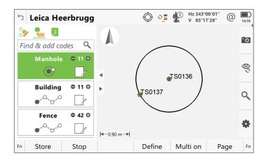
**3 pt circle (2D)** - using this linework option, a circle can be created by measuring three points on the circumference of the circle. The first measured point will define the height of the circle. Only three points will be exported, and other auxiliary points used to construct the shape will be hidden from view.
