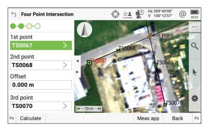
The renewed COGO app provides graphical confirmation of the complete calculation workflow, helping ensure the correct data is selected and the results are fully understood, reducing the chances to get unexpected results and saving time in the field.
