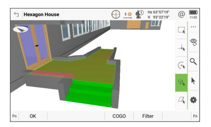
Additionally, when a face of an object is selected, the context menu offers a new option to use the selected face as a surface in the **Inspect Surfaces** app, where the surface can be compared to other surfaces or measurements.
