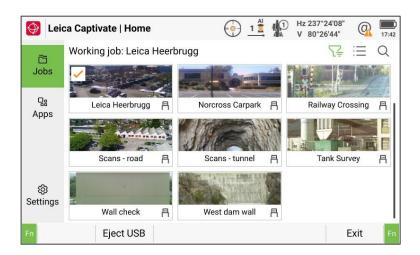
It is also possible to eject the USB stick once the side cover has been opened. Once the side cover is opened, a message will appear giving the option to **Eject USB**. The USB stick should only be removed after the orange confirmation message has appeared, informing that the USB stick is safe to remove.
