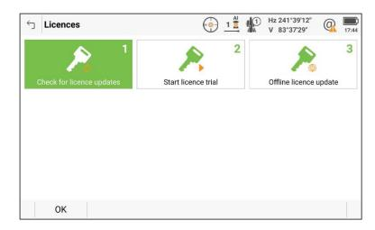
When the instrument is online, the licences can be checked and updated using **Check for licence updates**. Any changes to the licence will be automatically checked and applied. The licences are also automatically checked after startup once connected to the internet.
