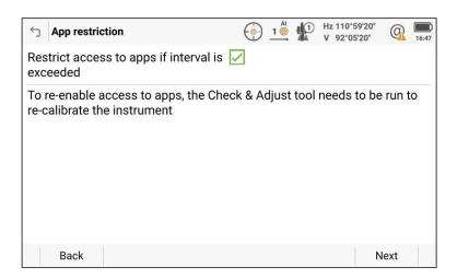
In addition, the **Restrict access** tool, found in **Settings/System**, has been extended to include the ability to restrict access to the **Check & Adjust settings**. Within the restrict access wizard, in the **TS settings** page, a new option to uncheck access to the check & adjust settings is introduced. By completing the **Restrict access wizard**, the user restrictions can be applied and a password set to secure access back into the user restrictions.
