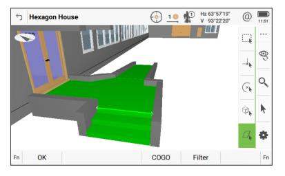
When the 'snap to face' tool is active, a face of a solid IFC object can be tapped to select the face of the object. The face selection is indicated by a green border and red-shaded fill. The context menu can then be opened to use object-specific tools such as importing the geometry or viewing IFC relevant information.
