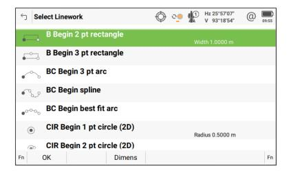
When moving the focus to either of the new linework rows, a new button **Dimens (F3)** appears, which leads to a panel allowing to edit the dimension of either the width of the rectangle, or the radius of the circle.
