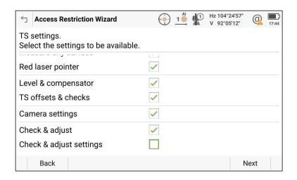
Together, these features allow, for example, an equipment or site manager to set up the workflow in a way that the site engineers using the instrument can only perform measurements with an up-to-date check and adjust calibration, providing a way of ensuring measurement quality control.
