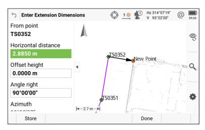
To support extending a line during coding & linework, a new hot key also allows extending the currently measured line without needing to select the line in the 3D Viewer. In the **Measure** app, when using codeboxes and the currently active codebox has linework in progress, pressing the button assigned to the hot key **User – Extend line** will open the **Enter Extension Dimensions** panel, as described previously.
