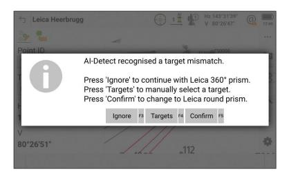
When a GMP111 or GMP111-0 Mini prism is detected, Al-Detect cannot differentiate between the two prism types, which have a similar appearance but different prism constants. In this case, the message will ask to confirm if the target is a **Mini** or **Mini-0** prism.
