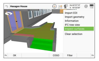
The new snapping tools allow selecting the specific items of interest when working with IFC data, meaning only those items need to be imported rather than the whole object. This keeps the data cleaner and makes it easier to work with.
