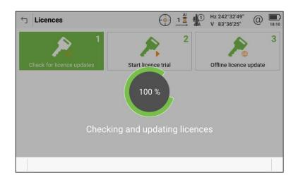
If the instrument is offline, it is also possible to update licences using **Offline licence update**. The wizard will guide through a series of steps, which involves generating a request file on the USB stick, uploading this on a PC to Leica MyWorld which will then send back a response file, and finally transferring this back to the instrument via the USB stick.
