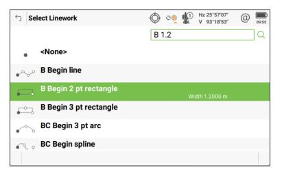
By confirming the selection with **OK (F1)**, the required points can then be measured and the linework will be created. In the example, measuring two points will define the rectangle length, and the dimension will define its width.
