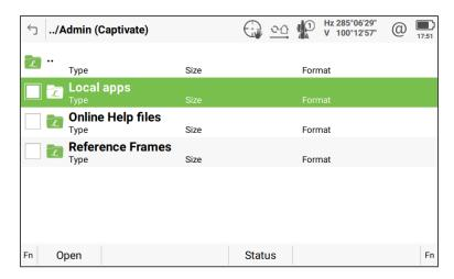
After choosing the appropriate device type folder, any number of apps can be selected and downloaded simultaneously. When the selected apps are downloaded, a message will appear, providing the option to go to the **Update Software** panel to accept the Software Licence Agreement and complete the install.
