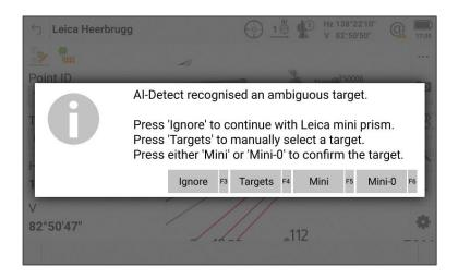
Al-Detect ensures measurements are made with the right prism type every time, reducing mistakes and ensuring data collection quality.
