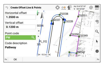
Note that if the selected line contains linework geometries including splines, clothoids, circles or rectangles, that it will not be possible to offset the line, and a warning message will appear.
