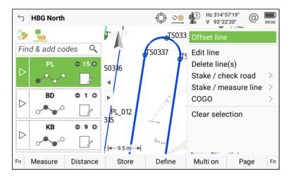
Selecting Offset line will open the Create Offset Line & Points panel, where the Horizontal offset and Vertical offset values can be entered. A new point code can also be assigned to the points of the offset line. The proposed offset line will be visible in the 3D Viewer, and the new line can be stored by pressing OK (F1).
