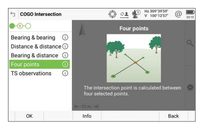
Once a sub-method is selected, the next split-screen panels allow selecting the points and entering the data for the calculation, as well as displaying the calculation results. The right side of the panel always shows the 3D Viewer, also allowing point selection and displaying the results graphically.
