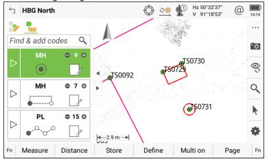
Having the ability to measure circles and rectangles with an input dimension speeds up data collection when measuring objects of known dimensions, whilst also providing flexibility if all corners of the feature cannot be measured.
